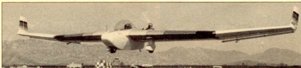
A poor man's Flying Wing, the Mitchell U-2 ultralight can ascend at 400 fpm or descend at a glide ratio of 25:1.
